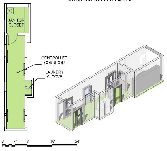
**Figure 3-11 Controlled Corridor Data Sheet**
