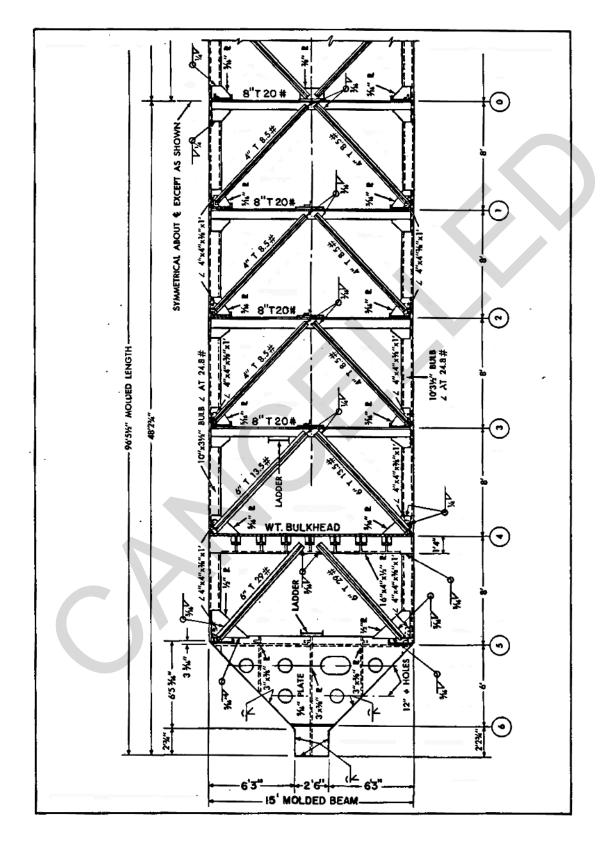
Fig. 9-2 Typical Horizontal Girder for Welded Caisson
