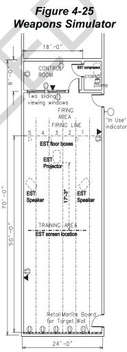
Ceiling – suspended acoustical ceiling tile (ACT). Ceiling to have 12" by 10" high raise notch along Simulator Room wall between Control Room and target wall for an exposed cable tray to be inserted. Top and side of raised notch shall be ACT.
