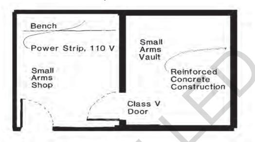
**4-5.3.2** A 110 volt continuous power strip should be provided over the work benches.
