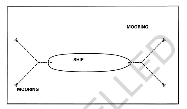
Figure 2-9. Bow-Stern Mooring Shown in Plan View
