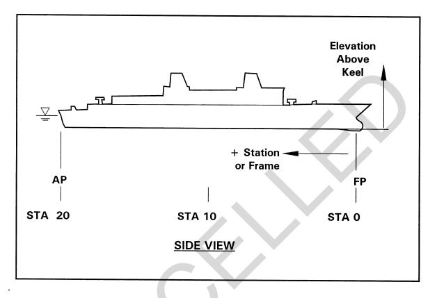
Figure 3-2. Ship Design and Hydrostatic Coordinates
