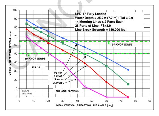
Six degree-of-freedom quasi-static analyses using the program AQWA LIBRIUM are performed on various LPD-17 mooring configurations to determine safe mooring limits as follows:
