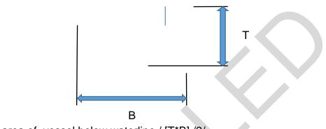
$C_m$  = Transverse area of vessel below waterline / [T\*B] /2/
