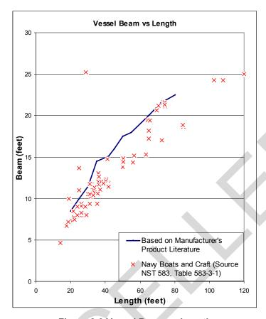
Figure 2-3 Vessel Beam vs Length
