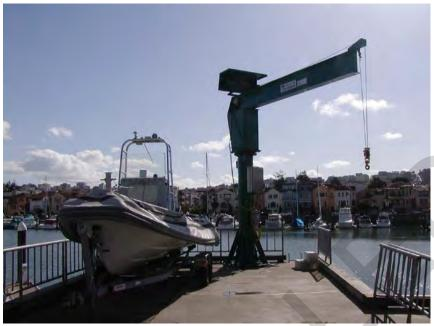
Figure 8-2, Small Craft Crane Access (Jib-boom)
