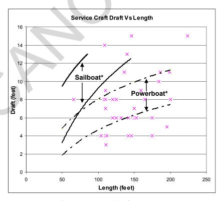
Figure 2-5 Vessel Draft vs Length
