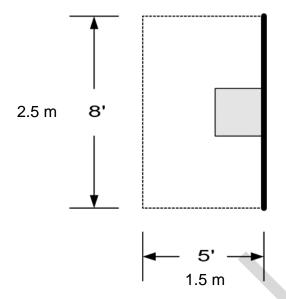
The workspace required around the cabinet is still required even if the cabinet is mounted 2.0 m (6.5 ft) off the floor.
