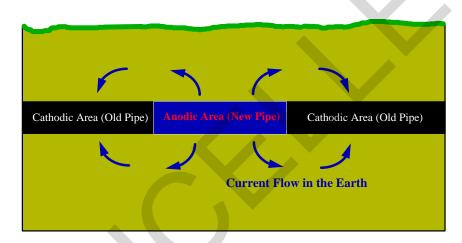
Figure 2-9. Galvanic Corrosion Cell Caused by Old and New Steel
