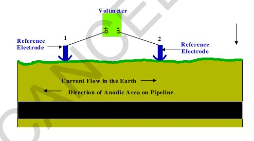
Figure 7-10. Positive Reading for Cell-To-Cell Survey
