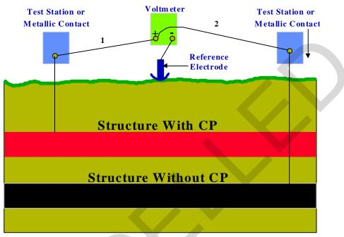
Figure 7-20. Testing For A Short Between Two Structures
