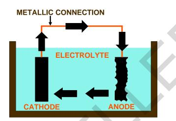
Figure 2-1. The Corrosion Cell
