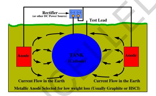
Figure 2-24. Impressed Current Cathodic Protection System
