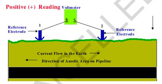
Figure 7-37. Cell-To-Cell Polarity on Foreign Structure
