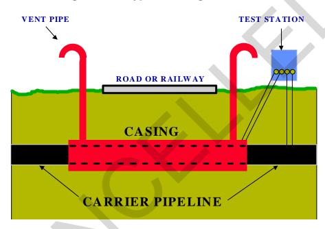
Figure 7-17. Typical Casing Installation
