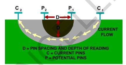
Figure 7-26. Soil Resistivity by the Four Pin Method (Wenner)
