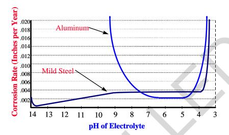
Figure 2-17. Effect of Electrolyte pH on the Rate of Corrosion
