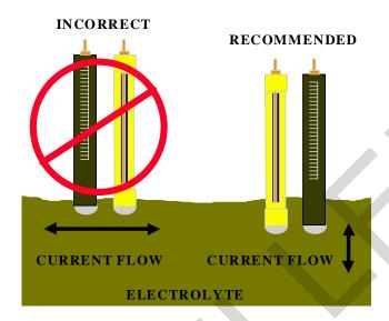
Figure 7-32. pH Measurement with Electrolyte Current Flow
