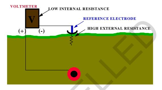
**Figure 7-4. Contact Resistance Error**
