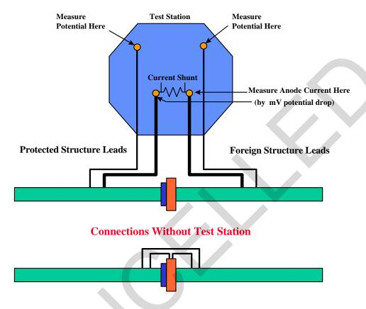
Figure 5-5. Bonding For Continuity
