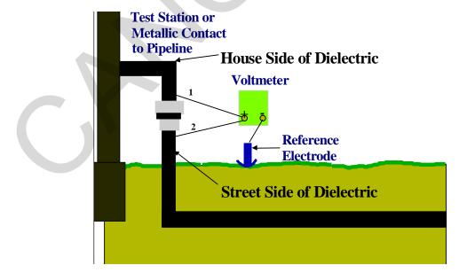
Figure 7-13. Testing for a Shorted Dielectric
