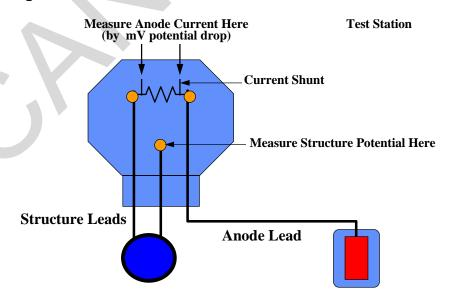
Figure 2-23. Potential - Current Test Station Connections
