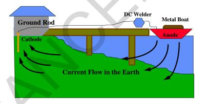
2-2.4.4 **Cathodic Protection Systems**. Cathodic protection systems are a major source of stray current on other metallic structures. An example of this electrochemical corrosion cell is when a foreign pipeline passes near an anode, and then crosses the protected structure (cathode). Detailed procedures are provided for testing and mitigation of these problems in Chapter 7.
