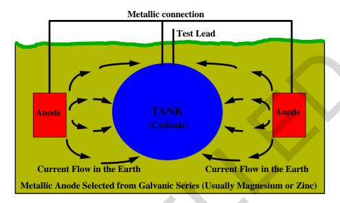
Figure 2-19. Distributed Sacrificial (Galvanic) Cathodic Protection System
