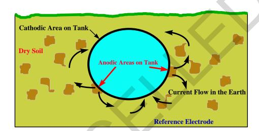
Figure 2-6. Concentration Cell Caused by Non-Homogeneous Soil
