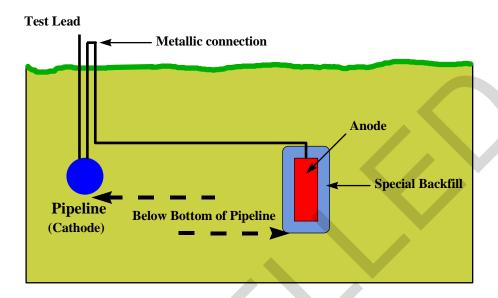
Figure 2-20. Galvanic Anode Installation
