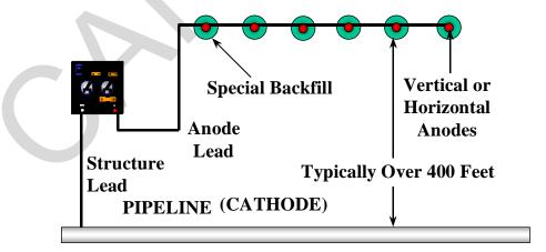
2-7.3.2 **Horizontal Remote Impressed Current CP Systems**. These systems are commonly used for pipelines in remote areas where a rock stratum is located near the surface or where other soil conditions would require horizontal installation to ensure the
