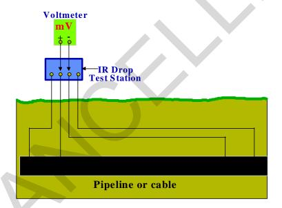
Figure 7-33. Typical IR Drop Test Span Installation
