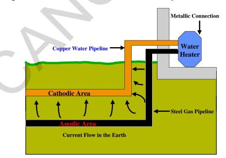
Figure 2-8. Galvanic Corrosion Cell Caused by Different Metals
