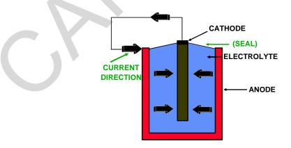
Figure 2-2. Corrosion Cell, The Dry Cell Battery
