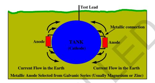
For the protection of underground structures such as pipelines, the anodes are not usually attached directly to the structure, but are placed in the soil, evenly distributed a short distance from the pipeline, and are connected to the pipeline by a wire, usually through a test station. This type of sacrificial anode system is shown in Figure 2-19.
