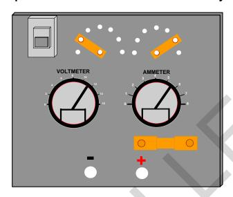
Figure 2-25. Impressed Current Cathodic Protection System Rectifier
