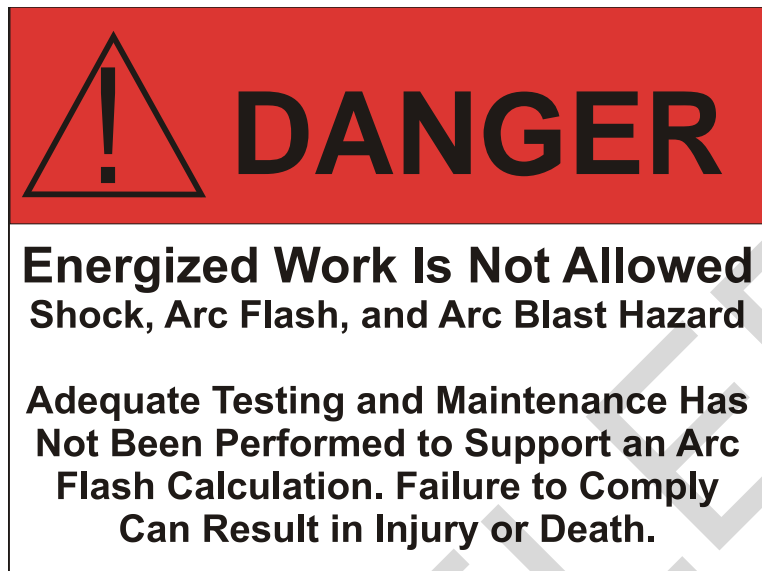
Figure 1-10 Arc Flash Danger Label for Equipment Without Documented Maintenance and Testing
