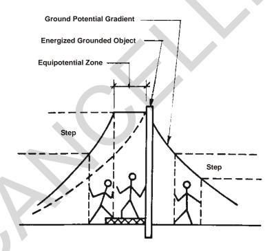
Figure 1-1. Ground Potential Gradient
