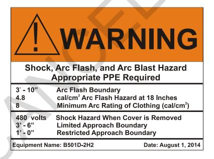
Figure 1-8 Typical Detailed Arc Flash Warning Label Showing Site-Specific PPE
