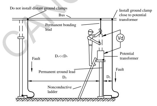
Figure 7-1. Substation Temporary Grounding
