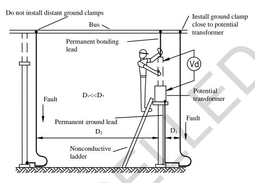
Figure 7-1. Substation Temporary Grounding
