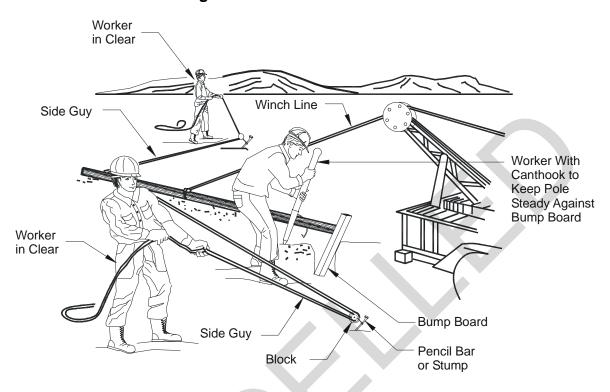
Figure 10-2. Winch Line Method
