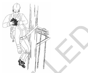
Figure 14-3. Position to Support Victim's Body Weight
