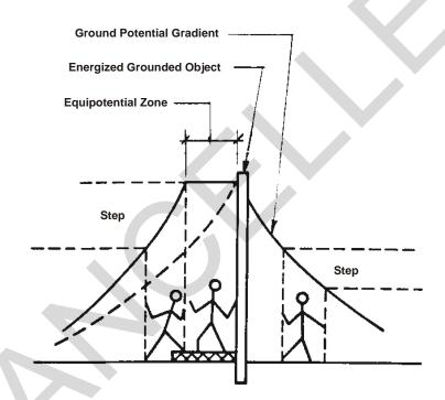
**Figure 1-1. Ground Potential Gradient**
