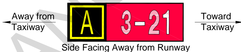
LOCATION SIGN COLLOCATED WITH RUNWAY HOLD SIGN
