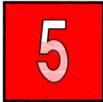
RUNWAY HOLD SIGN (AT END INTERSECTION)
