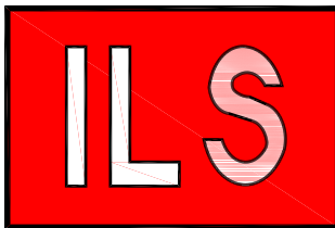
HOLD SIGN AT ILS CRITICAL AREA
