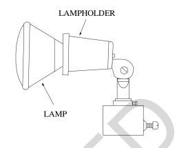
Figure 13-7. FAA-L-850B, In-pavement, Uni-directional
