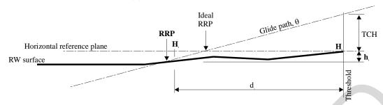
Use this method if longitudinal runway grade changes within 671 meters (2200 feet) from the runway threshold. Consider that a 0.1% <u>change</u> in runway grade at about 150M (500') from threshold translates to a 15cm (6") change in elevation at 300M (1,000'), and about a 3M (10') error in calculating the RRP, using the runway grade beginning at the threshold. The trial method requires elevation data along the runway centerline in proximity of the PAPI site.
