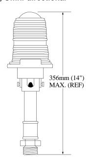
Figure 13-13. FAA L-852, (A, B, C, D), In-pavement, Bi-directional
