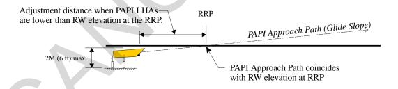
B. When lens is **above** RW elevation at RRP.
