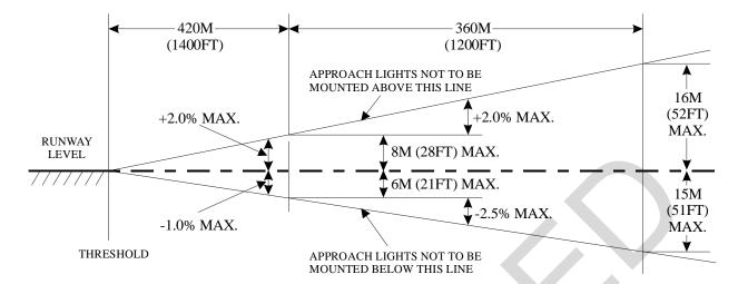
Figure 3-10. Light Plane Elevation Limits
