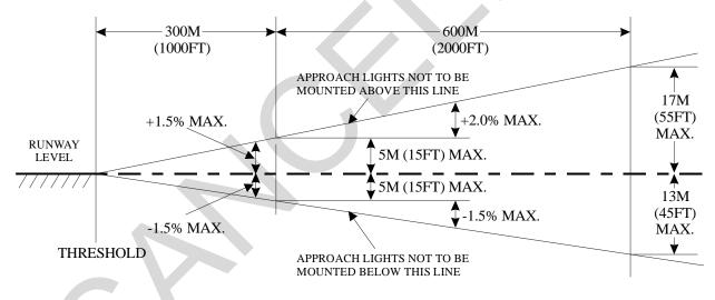
Figure 3-3. Light Plane Elevation Limits
