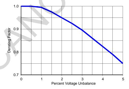
Figure C-1 Typical Derating Factor for Three-Phase Induction Motors
