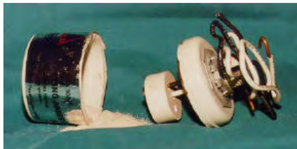
Figure D-2. Unlisted Surge Protector
