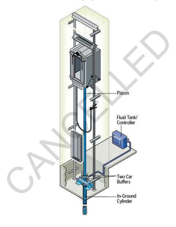
Figure B-3 Hole-less, Dual Post, Direct Plunger Hydraulic Elevator
