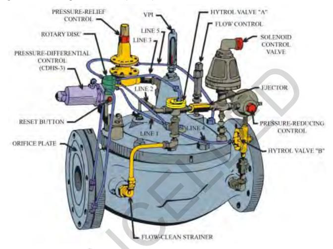
Figure 5.4. Refueling Control Valve (90AF-8).
