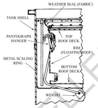
Figure 7.5. Floating Pan Detail.
