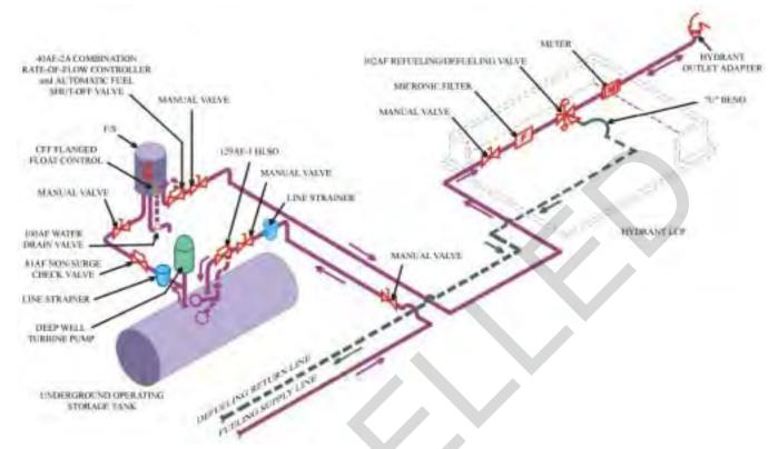
Figure 4.1. Modified Panero, Type I Hydrant System.
