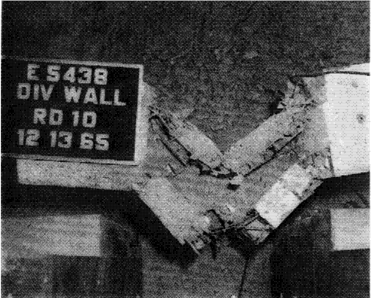
Figure 4-6 Failure of a Laced Element
