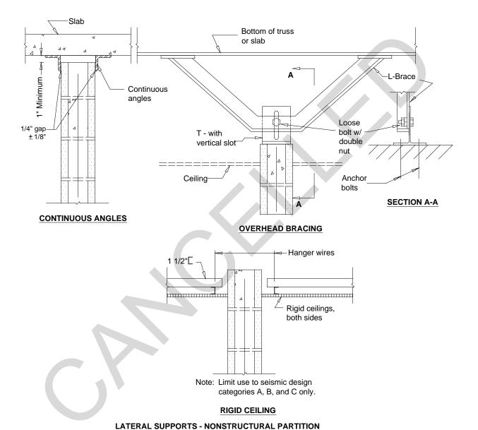
Figure B-2. Typical Details for Isolation of Rigid Partition Walls
