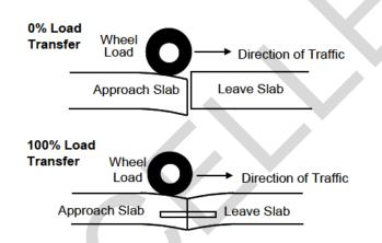
Figure 18-1 Load Transfer at a Joint
