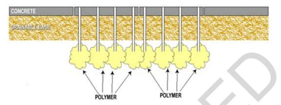
Figure 15-2 The Polymer Deep Injection Process
