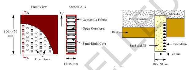
Figure 19-2 Geocomposite Edge Drain Features & Installation Details
