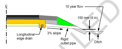
Figure 19-4 Outlet Pipe Design
