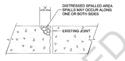
Figure 12-12 Existing Partial-depth Spalled Joint
