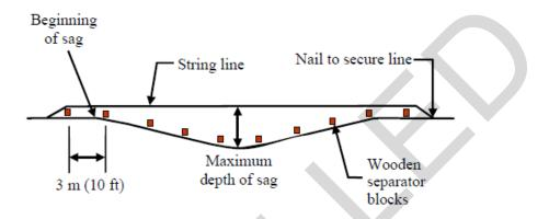
Figure 15-4 Elevation Control
