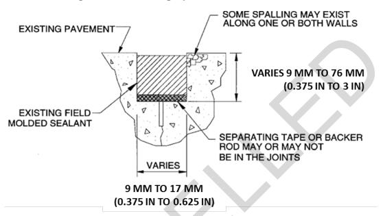
Figure 12-9 Existing Spalled Field Molded Joint
