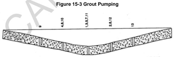
PUMPING STARTS AT LOWEST POINT AND WORKS OUTWARD IN BOTH DIRECTIONS
