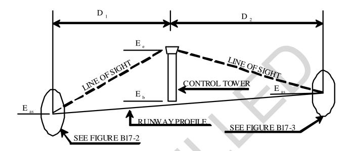
Figure B17-2. Minimum Eye-Level Determination
