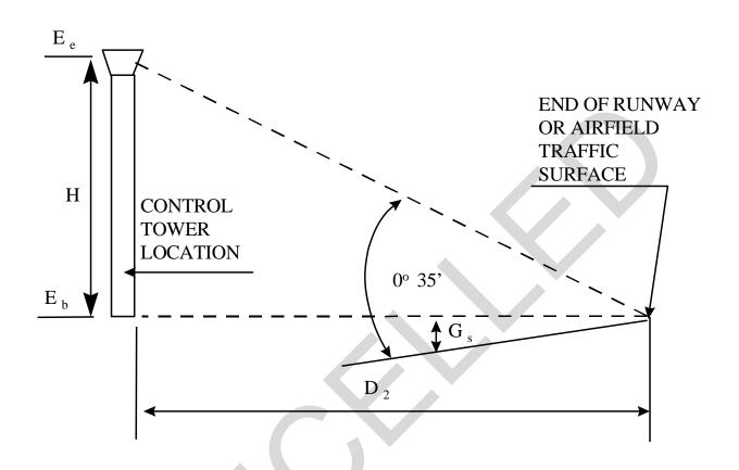
Given: E  $_{as}$  = 33.5 m (110') MSL E  $_{b}$  = 32.3 m (106.0') MSL D  $_{2}$  = 1,828.8 m (6,000')
