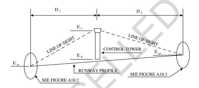
Figure A18.2. Minimum Eye-Level Determination.
