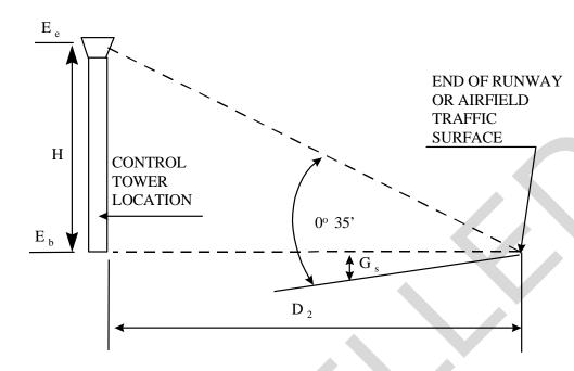
Given:  $E_{as} = 33.5 \text{ m} (110') \text{ MSL E b} = 32.3 \text{ m} (106.0') \text{ MSL}$
