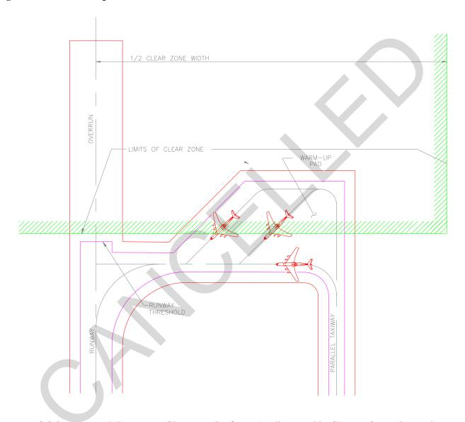
6.8.3.2. Approach Departure Clearance Surface. As discussed in Chapter 3, an obstruction to air navigation occurs when the imaginary surfaces are penetrated. Do not site warm-up pads, other aprons, hot cargo spots, or taxiways to these facilities in a way that will allow penetration of the Approach Departure Clearance Surface. Such aircraft penetrations may require revisions to TERPS procedures. Properly sited warm-up positions are illustrated in Figure 6.12.
