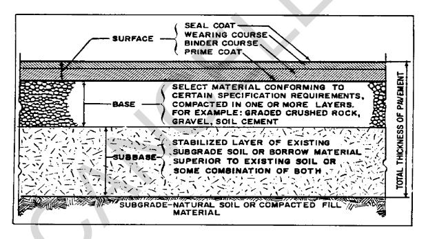
FIGURE 1 Flexible Pavement Terminology
