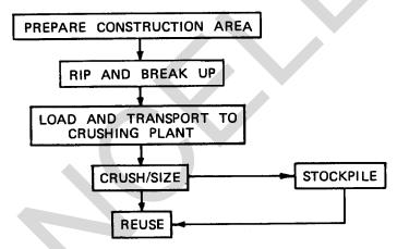
Figure 5-1. Recycling portland cement concrete flow process.
