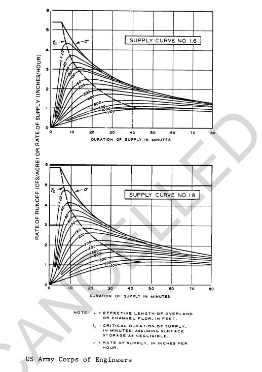
Figure B-10. Rates of runoff corresponding to supply curves No. 1.6 and 1.8; n = 0.40 and S = 1 percent.
