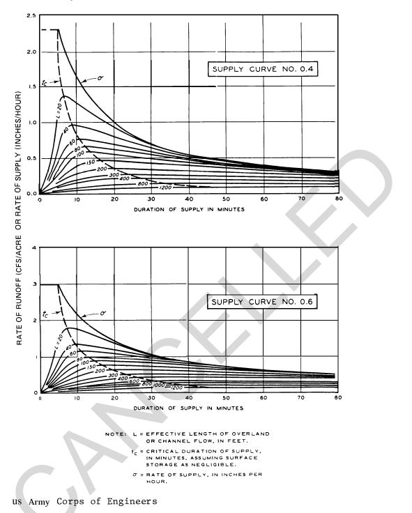
Figure B-7. Rates of runoff corresponding to supply curves No. 0.4 and 0.6; n = 0.40 and S = 1 percent.
