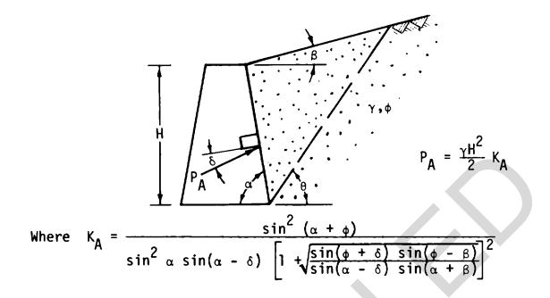
$\therefore$  Component of  $\mathsf{P}_{A}$  perpendicular to wall back is:
