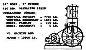
DESIGN CRITERION : SNOOTH OPERATION ( LESS THAN 0.10 IN / SEC VELOCITY ) At 450 RPM THIS REQUIRES  $A_{\rm E} = 0.002$  IN.
