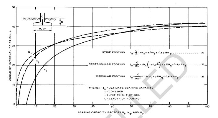
Figure 6-1. Ultimate hearing capacity of shallow foundations under vertical, eccentric loads.
