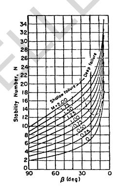
Figure 8-6. Stability charts for infinite slopes.
