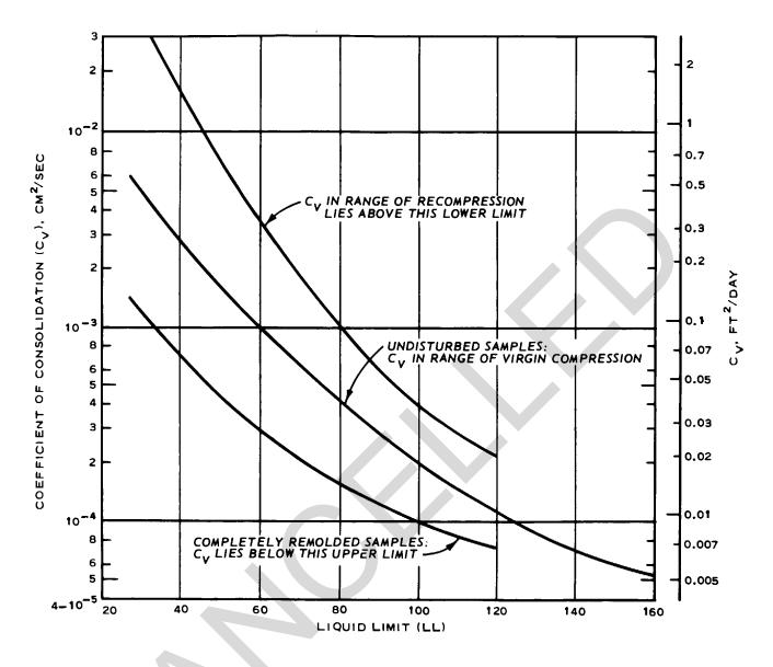
Figure 3-11. Correlations between coefficient of consolidation and liquid limit.
