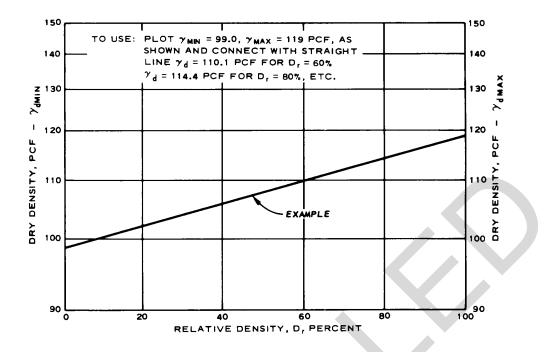
Figure 3-2. Relation between relative density and dry density (scaled to plot as a straight line).
