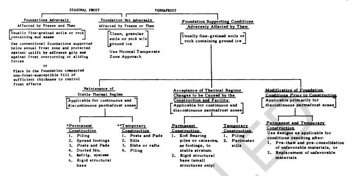
\*Permanent Construction - Construction incorporating the type and quality of materials and equipment, and details and methods of construction, which results in a building or facility suitable to serve a specific purpose over a minimum life expectancy of 25 years with normal maintenance.
