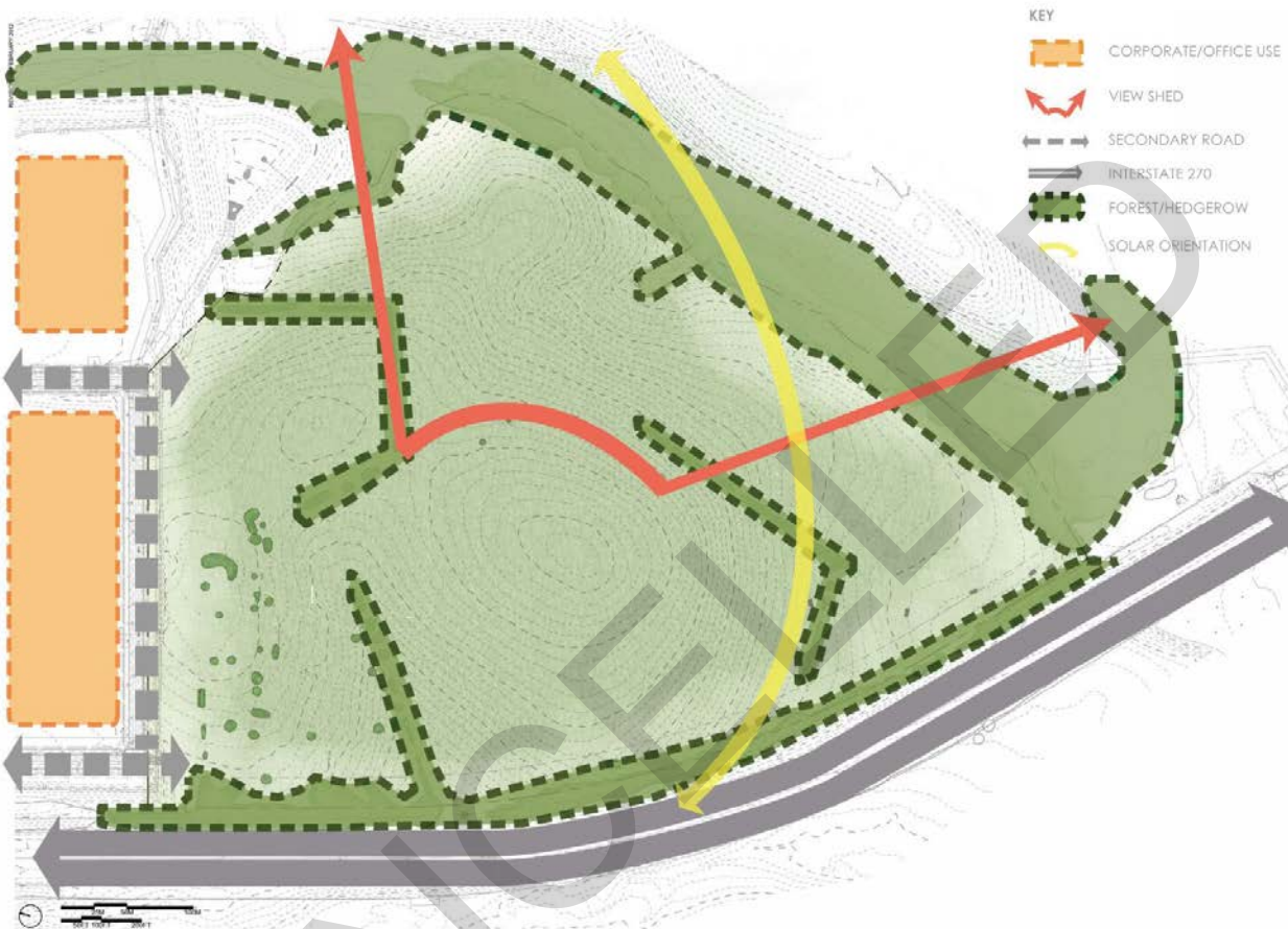
Figure 3-1 (Cont'd) Examples of Site Analysis Plans Land Use, Viewsheds, and Solar Aspect
