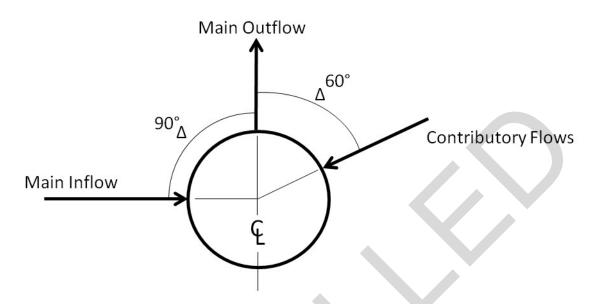
g. Provide a structure at collection and inlet points, at changes in horizontal or vertical alignment, at pipe junctions and with minimum spacing of a pipe run according to Table 3-1. Provide a discharge structure wherever flow changes from piped to open channel flow.
