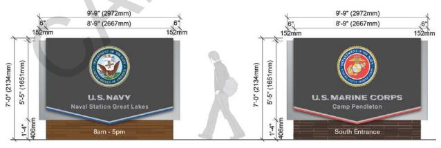
Figure 3-7 Secondary Installation Identification Signs.
