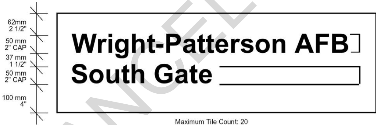
Figure 4.10. Entry Gate Type A3 Expanded Layout.
