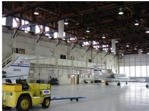
Figure C-7 Example of Clerestory Application
