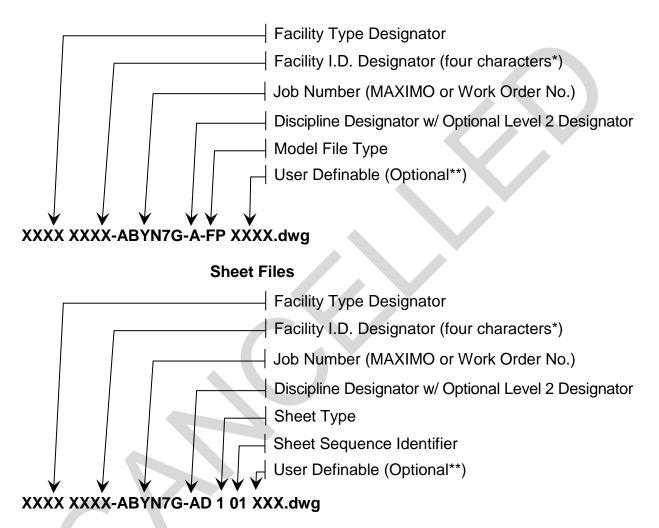
\* If no building designation has been assigned, such as for new construction prior to completion, then utilize the project number (P-number) for the Facility Type and I.D. designators. If installation has an alternate building identification system, that designator may be utilized in lieu of the Facility Type and Facility I.D. Designator.
