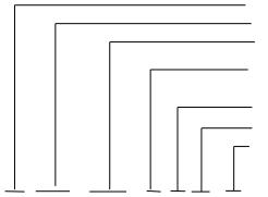
Fiscal Year of Construction Contract Construction Contract Number Task Order Number (if Applicable) Discipline Designator w/optional Level 2 Designator Sheet Type Sheet Sequence Identifier Record Drawing Suffix
