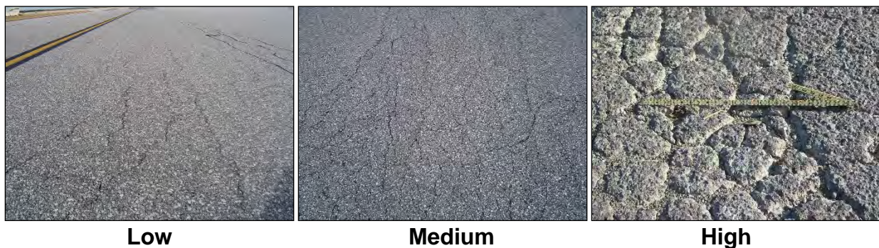
Figure B-1 Alligator Cracking Severity Levels
