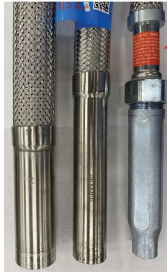
Figure 3-19 Comparison of Welded and Adjustable Reducers for Connections of Sprinklers to The Flexible Hose (Courtesy of TERPconsulting)
