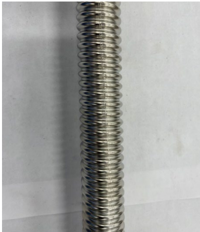
Figure 2-4 Example Corrugated Unbraided Helical Flexible Hose (Courtesy of TERPconsulting)
