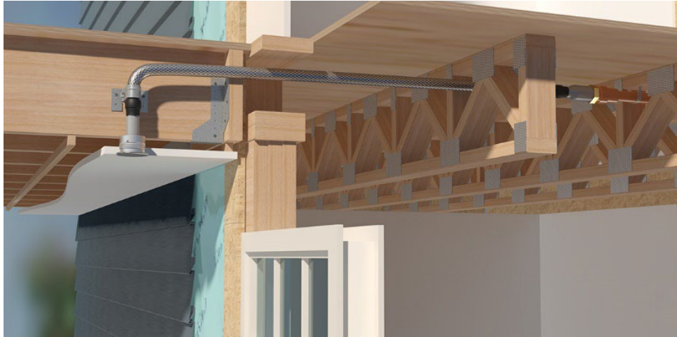
Figure 3-8 Dry Pendent Sprinkler Installation (Courtesy of Victaulic)
