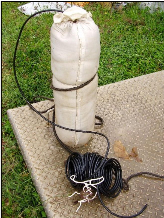
Figure 7 Packaged magnesium anode with outer paper wrapping removed.
