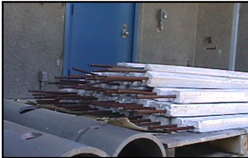
Figure 2 50 LB zinc anodes with steel cores for use in seawater.
