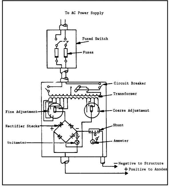
Figure 12 Single Phase, Full-Wave Bridge Rectifier
