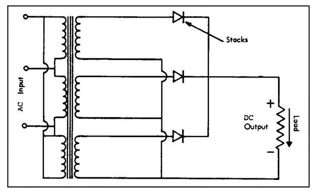
Figure 16 Three-Phase Wye Circuit Schematic
