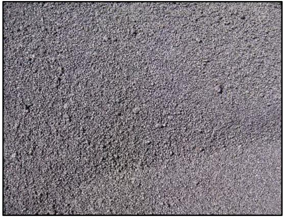
Figure 10 Petroleum coke backfill
