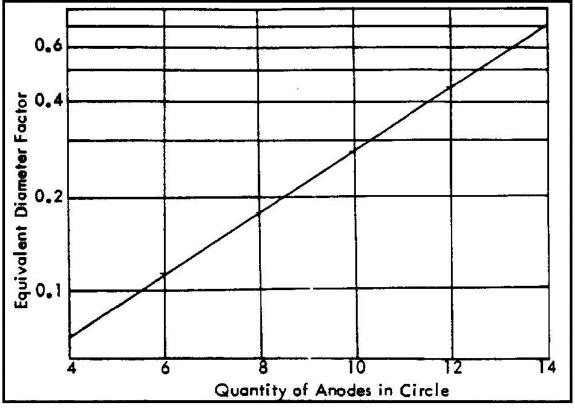
Figure 44 Equivalent Diameter for Anodes in a Circle in a Water Tank
