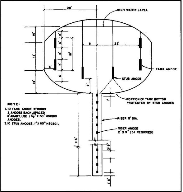
Figure 43 Anode Suspension Arrangement for Elevated Steel Water Tank
