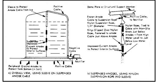
Figure 30 Impressed Current CP for Small Water Tank
