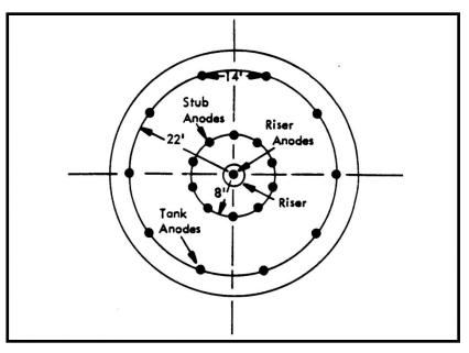
Figure 42 Anode Spacing for Elevated Water Tank
