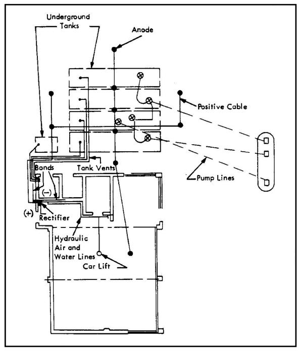
Figure 38 Impressed Current CP System for a Gasoline Service Station
