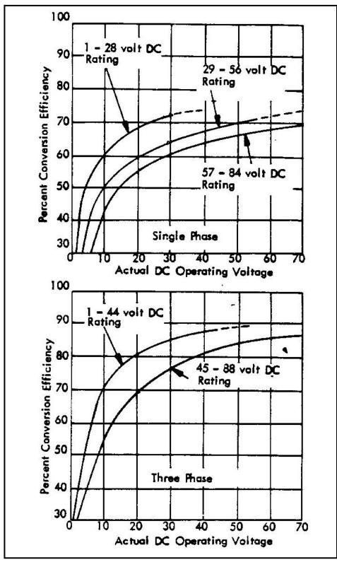
Figure 23 Efficiency versus voltage for selenium stacks
