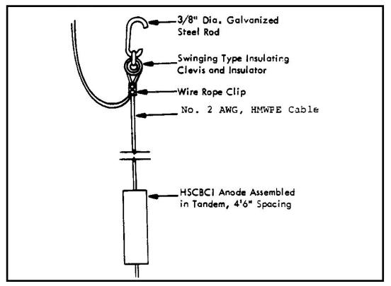
Figure 48 Riser Anode Suspension Detail for Elevated water Tank
