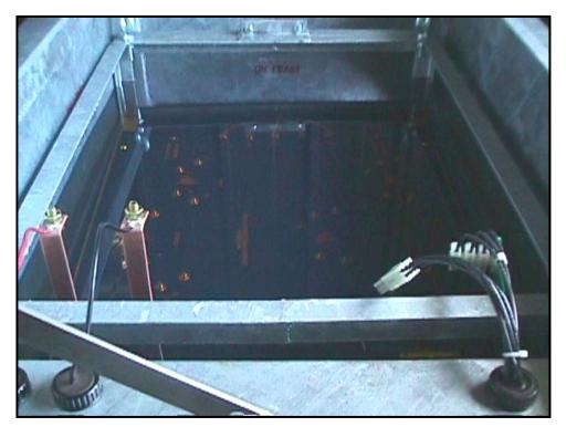
Figure 21 Typical entirely immersed oil-cooled rectifier.
