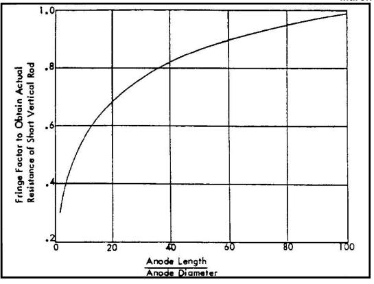
Figure 45 Fringe Factor for Stub Anodes
