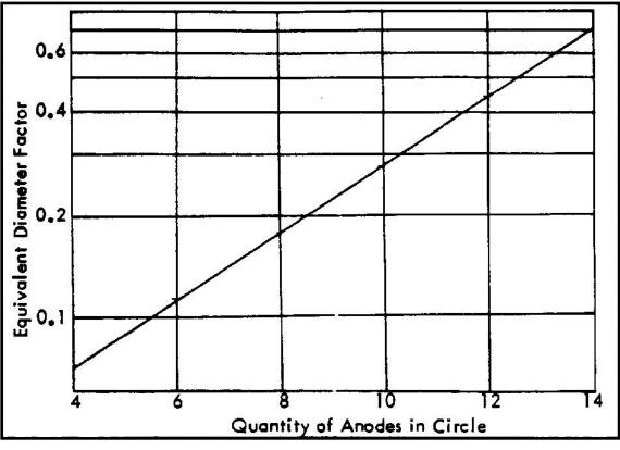
Figure 44 Equivalent Diameter for Anodes in a Circle in a Water Tank
