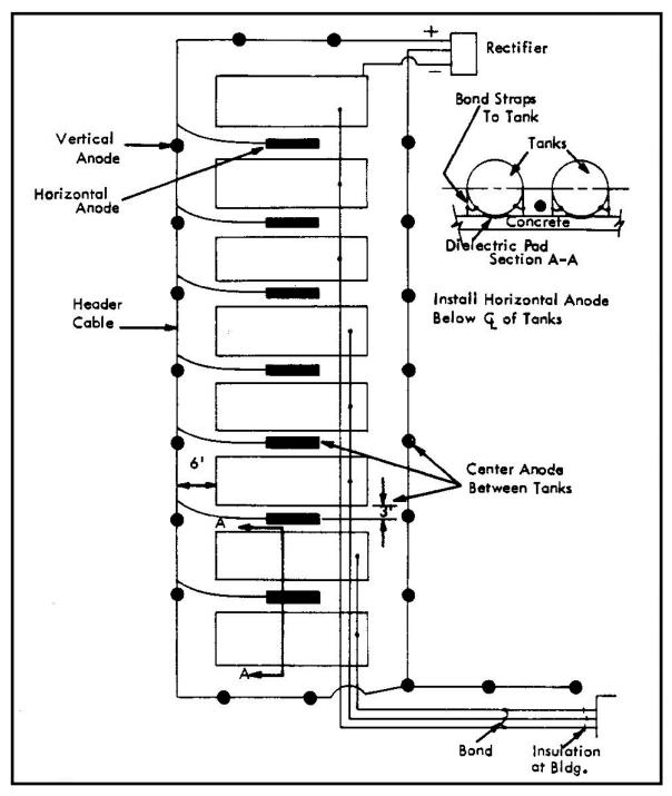
Figure 37 Typical Distributed Anode Impressed Current CP for Underground Storage Tank Farm
