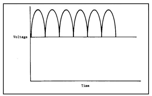
Figure 13 Full-Wave Rectified Current
