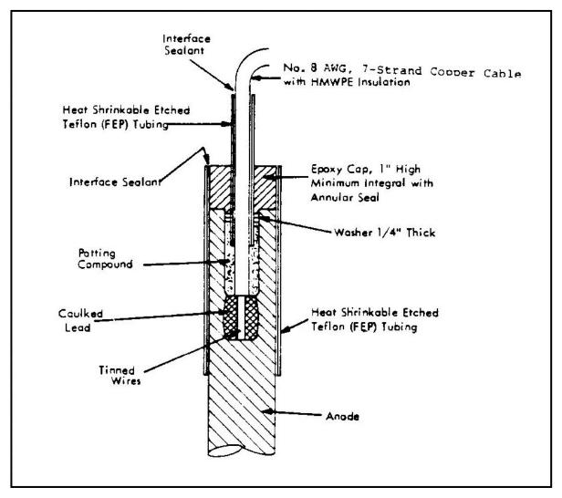
Figure 2 Anode to cable connection – Teflon seal.
