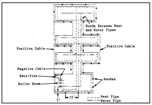
Figure 25 CP for Building Underground Heat and Water Lines
