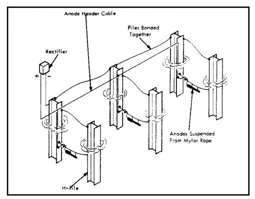
Figure 33 Suspended Anode Impressed Current CP for H-Piling in Seawater
