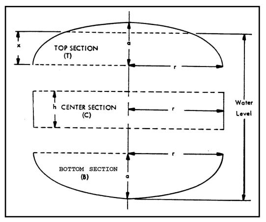
Figure 41 Segmented Elevated Tank for Area Calculations
