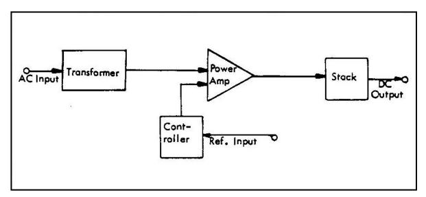
Figure 19 Constant Potential Rectifier Block Diagram
