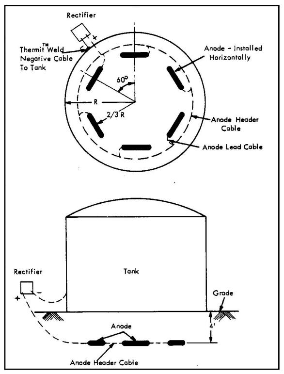
Figure 29 Impressed Current CP with Horizontal Anodes for On-Grade Storage Tank
