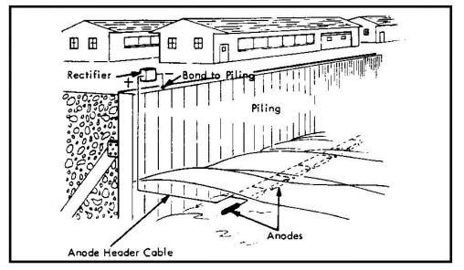
Figure 32 Impressed Current CP with Distributed Anodes for Water Side of a Steel Sheet Pile Bulkhead Wall
