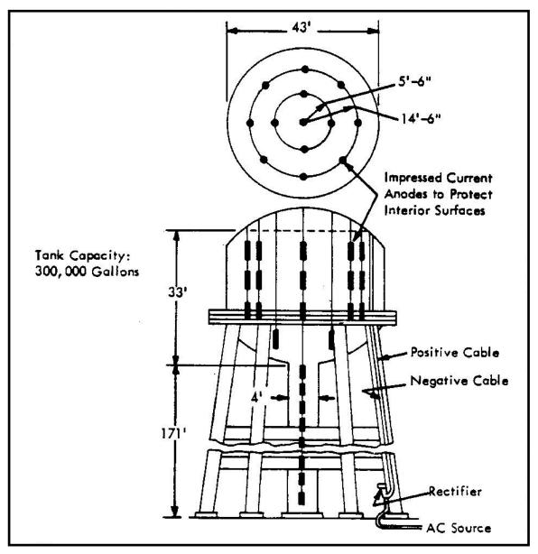
Figure 36 Impressed Current CP for Elevated Water Storage Tank Interior
