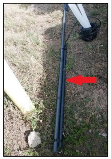
Figure 9 Mixed Metal Oxide tubular anode.
