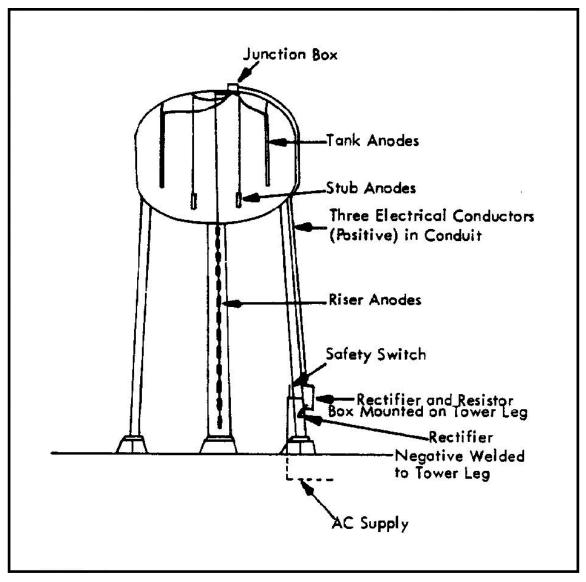
Figure 46 Elevated Steel Water Tank Showing Rectifier and Anode Arrangement
