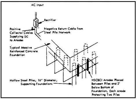
Figure 27 Cathodic Protection of Foundation Piles
