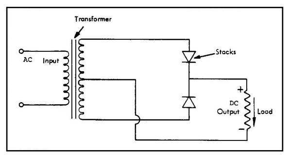
Figure 14 Single-Phase Center-Tap Circuit
