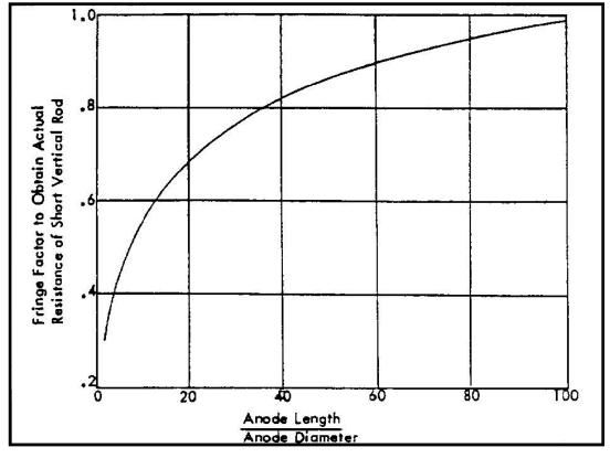
Figure 45 Fringe Factor for Stub Anodes
