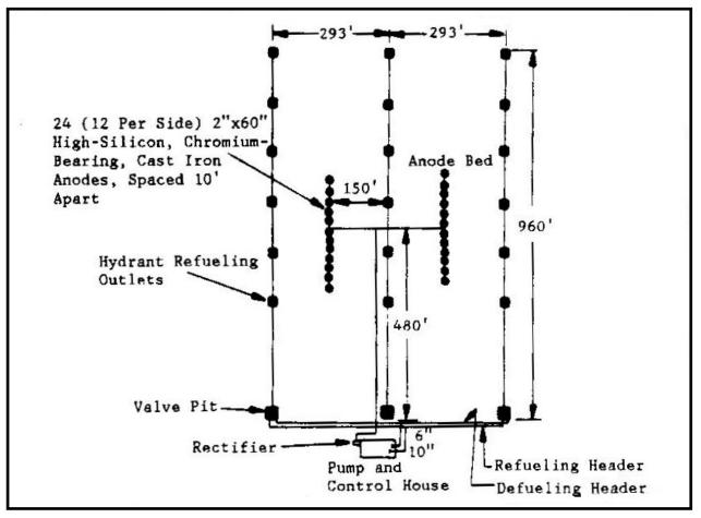
Figure 26 Impressed Current Type CP System for Aircraft Hydrant Refueling System
