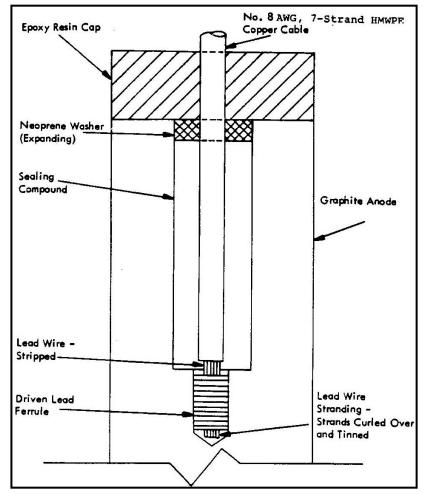
Figure 1 Typical anode end connection and seal
