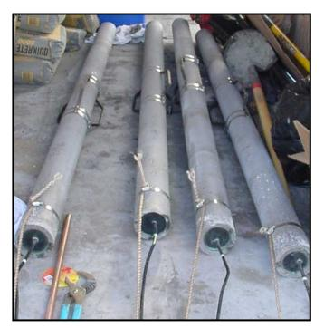
Figure 5 Tubular HSCBCI Anodes
