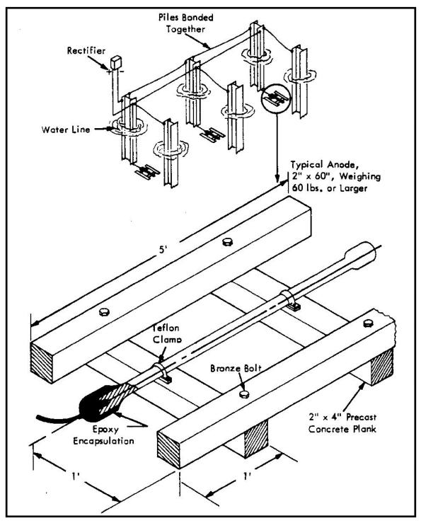
Figure 34 Impressed Current CP Sled Anode for H-Piling in Seawater
