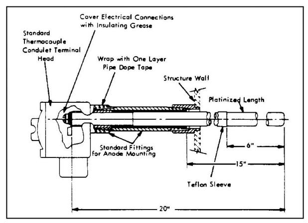
Figure 6 Example platinized anode configuration
