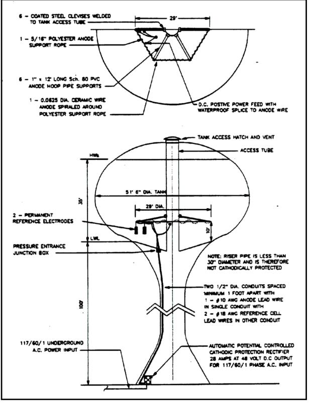
Figure 49 Elevated Pedestal tank with ceramic anode wire ring for icing conditions.
