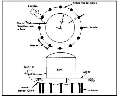
Figure 28 Impressed Current CP for Existing On-Grade Storage Tank
