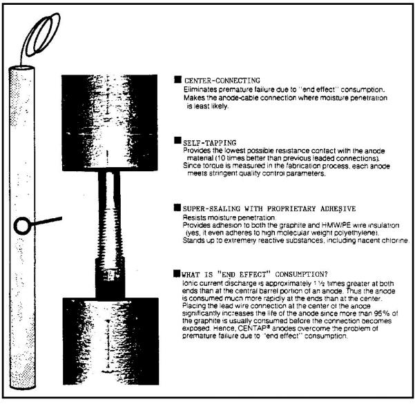
Figure 1a Center Connected Graphite Anode
