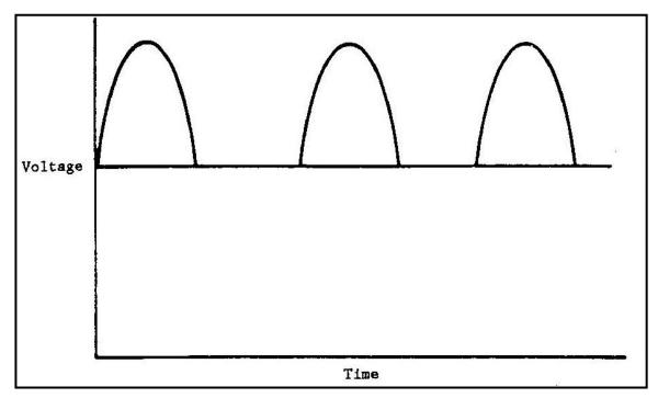
Figure 17 Half-wave rectifier output
