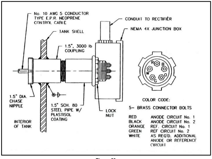
Figure 50 Pressure entrance fitting for underwater power and reference electrode wire penetrations in water storage tanks. 5.6 **Steel Gas Main.** Design an impressed current cathodic protection system for the 6-inch welded steel gas main shown in Figure 51. The pipeline has not yet been constructed, so current requirement tests cannot be conducted.
