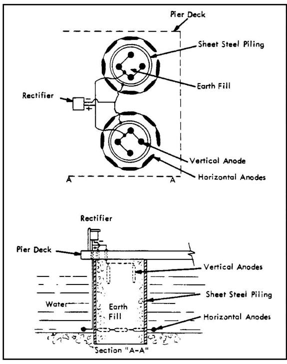
Figure 35 Impressed Current CP for Cellular Earth Fill Pier Supports
