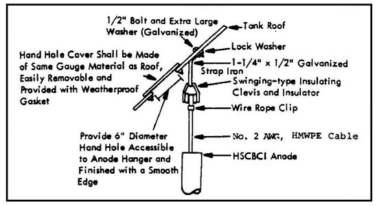
Figure 47 Hand Hole and Anode Suspension Detail for Elevated Water Tank
