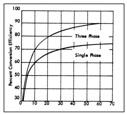
Figure 24 Efficiency versus voltage for silicon stacks
