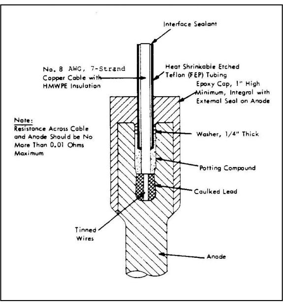
Figure 3 Anode to cable connection – Epoxy seal.
