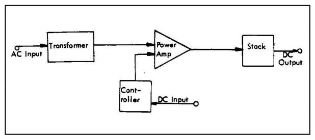
Figure 18 Constant Current Rectifier Block Diagram
