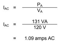
One 15 or 20 ampere circuit breaker in a nearby electrical panel will be sufficient.
