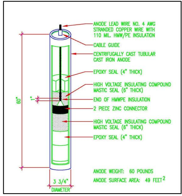
Figure 4 Anode to cable center connection
