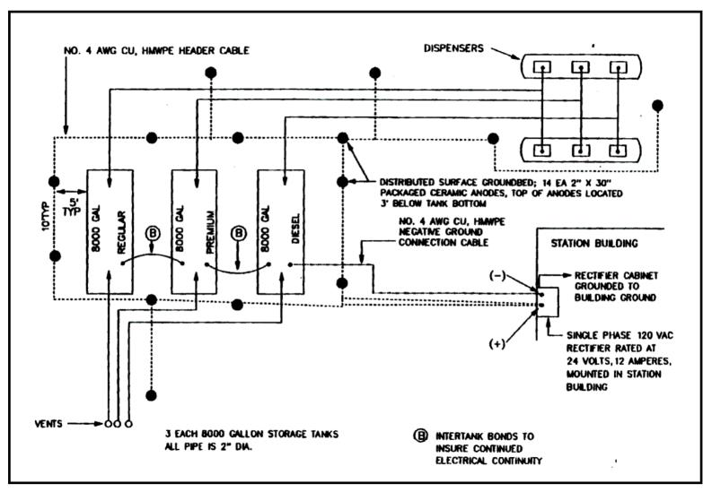
Figure 40 Cathodic Protection of Multiple Underground Storage Tanks
