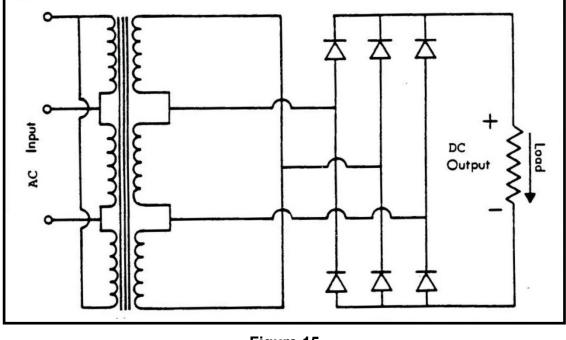
Figure 15 Three-Phase Bridge Circuit
