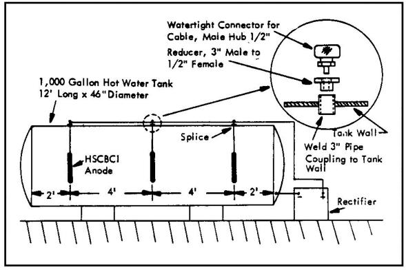
Figure 52 Cathodic Protection for an Industrial Hot Water Storage Tank
