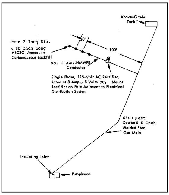
Figure 51 Cathodic Protection System for Gas Main
