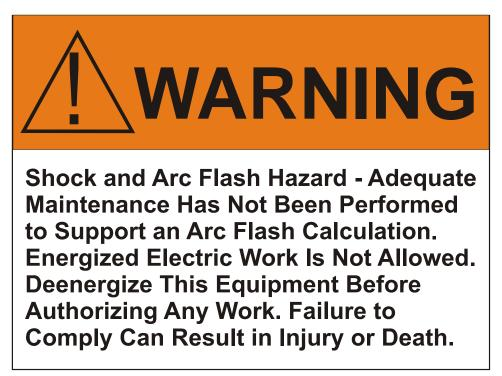
Figure 13 Arc Flash Warning Label if Maintenance and Testing Is Not Performed
