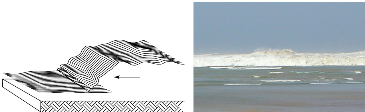
Figure 2-5 Sketch of a bore and photo from the 1983 Nihonkai-Chubu tsunami showing the formation of a bore offshore (photo from Knill and Knill, 2004).
