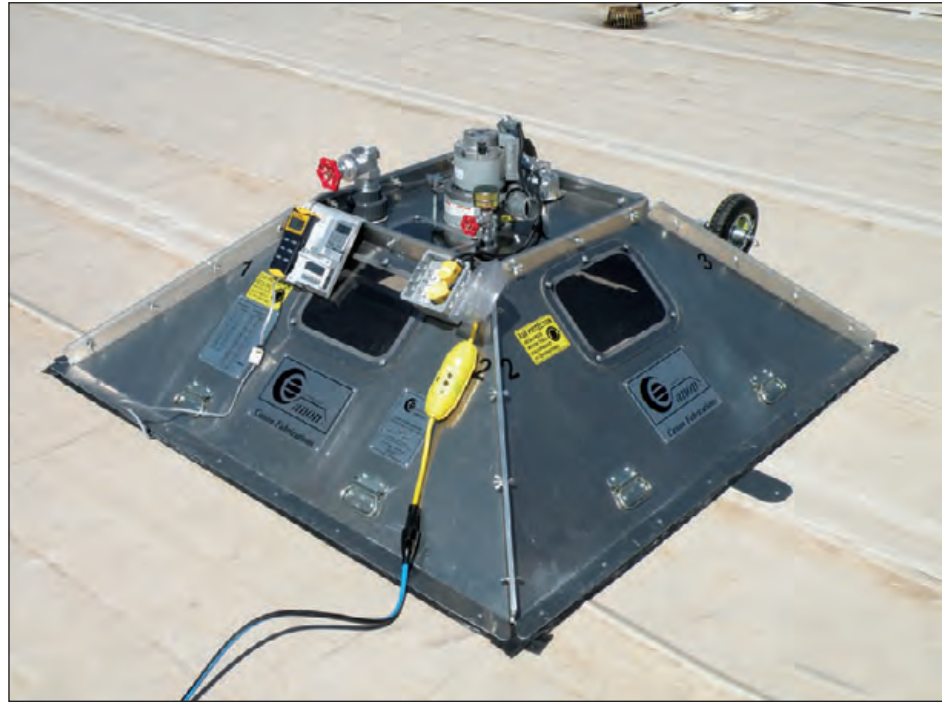
Figure 6-130: View of a 5-foot by 5-foot negative pressure chamber used to evaluate roof system uplift resistance.
