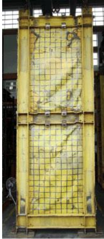
Figure 1.5-6 SPSW After Testing to Nearly 5% Drift (Li et al., 2009)
