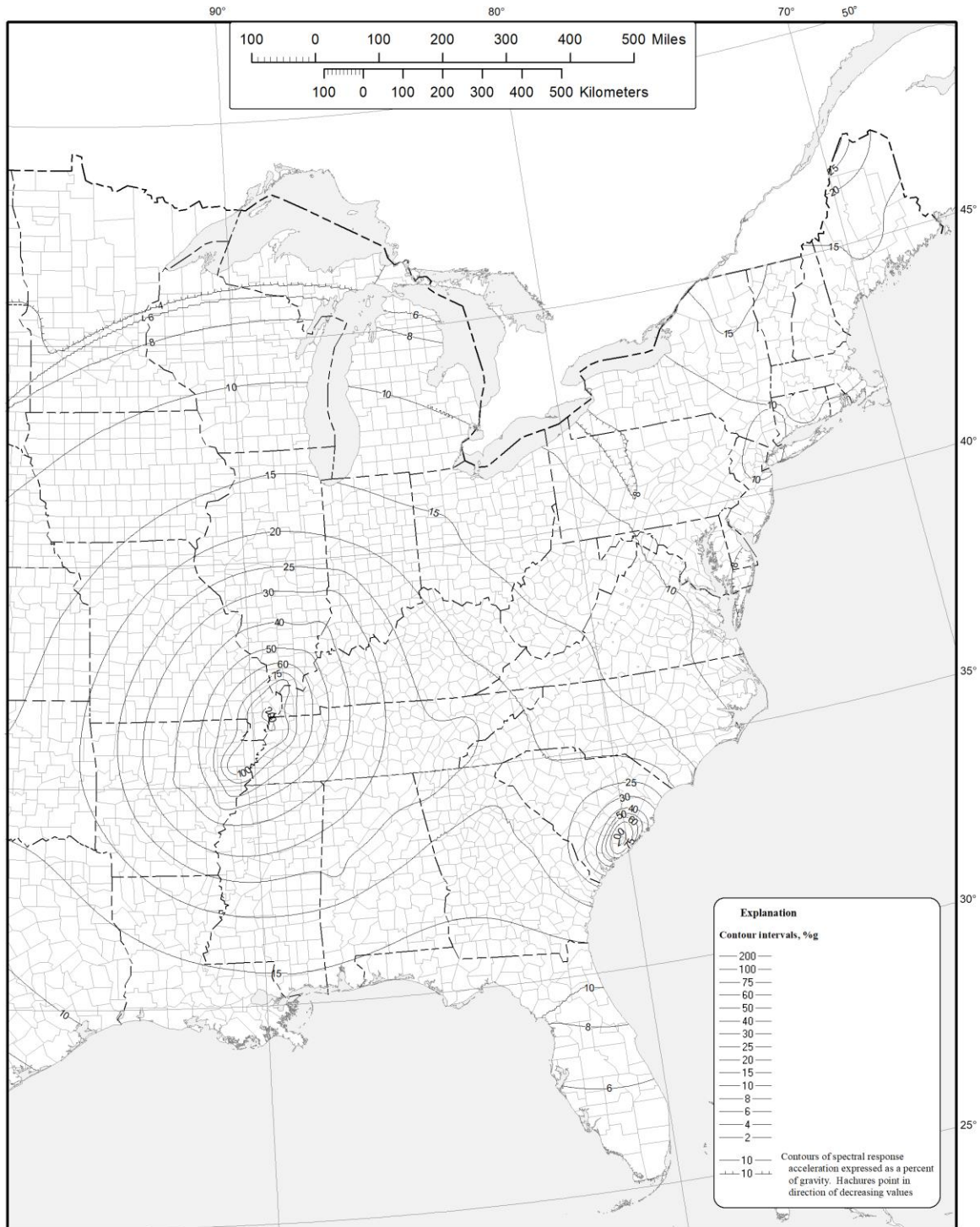
Figure 22-2 (continued) S_{M1} for the Default Site Class, for the Conterminous United States
