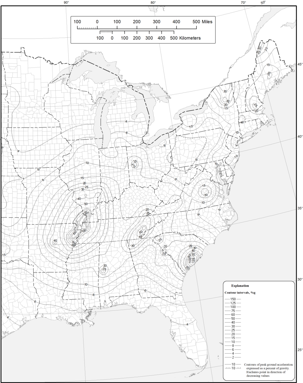
Figure 22-9 (continued) PGA_M for the Default Site Class, for the conterminous United States
