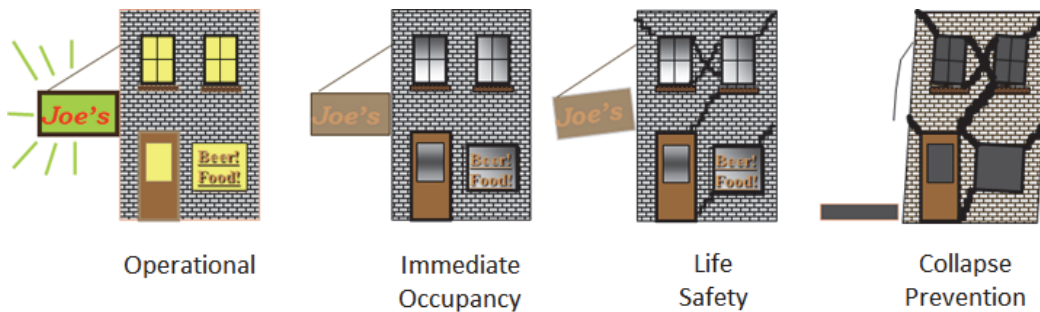
Figure 10-1 Standard ASCE/SEI 41 performance levels.
