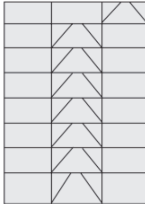
Figure 8-9 Example of an in-plane discontinuity irregularity.
