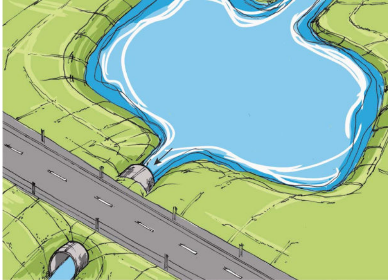
Figure 1.3.19. A sediment basin can help settle suspended sediment and decrease culvert clogging potential.
