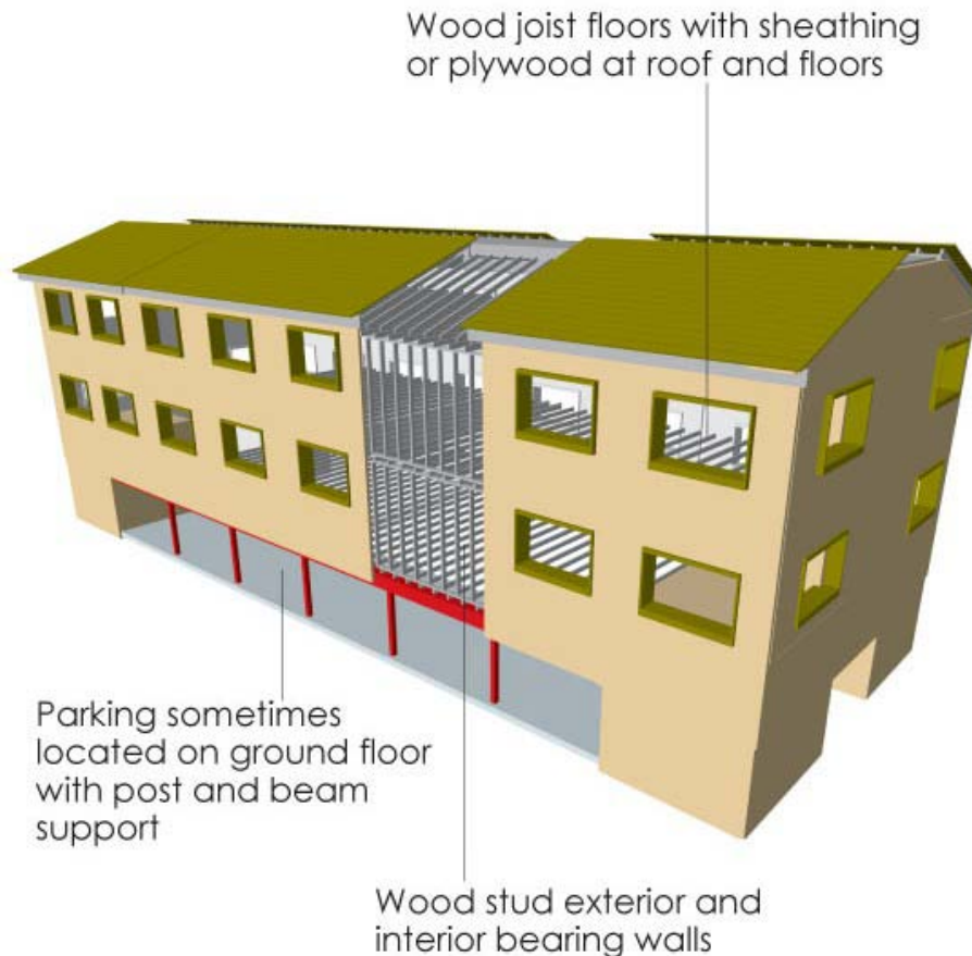
Figure 6.1-1: Building Type W1A: Multistory Multi-Unit Residential Woodframes
