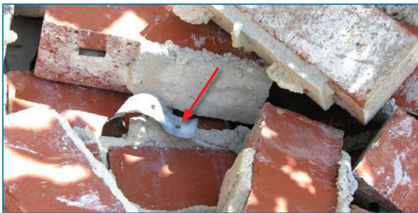
Figure 3-46: This tie remained embedded in the mortar joint while the smooth-shank nail pulled from the stud.
