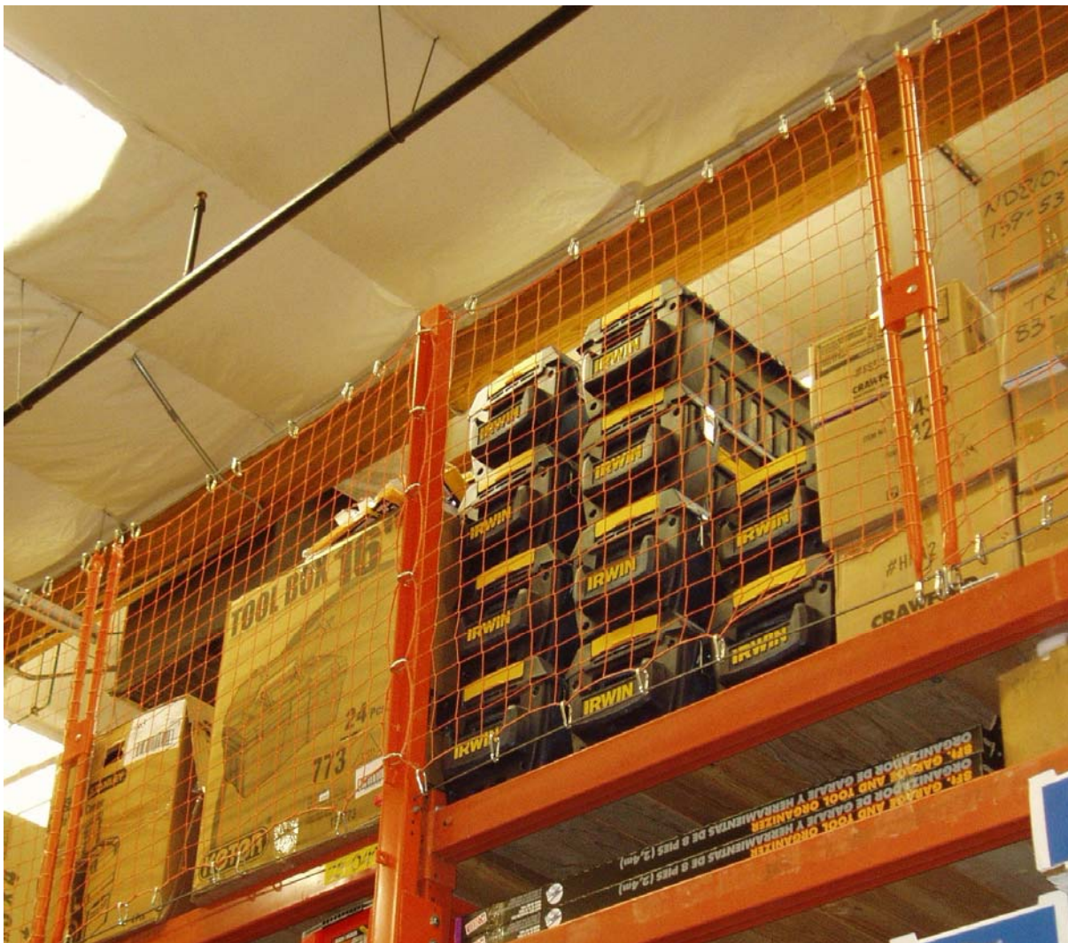
Figure 8-5 Merchandise restrained by netting.
