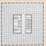
Plan of reinforced concrete shear wall building with center core
