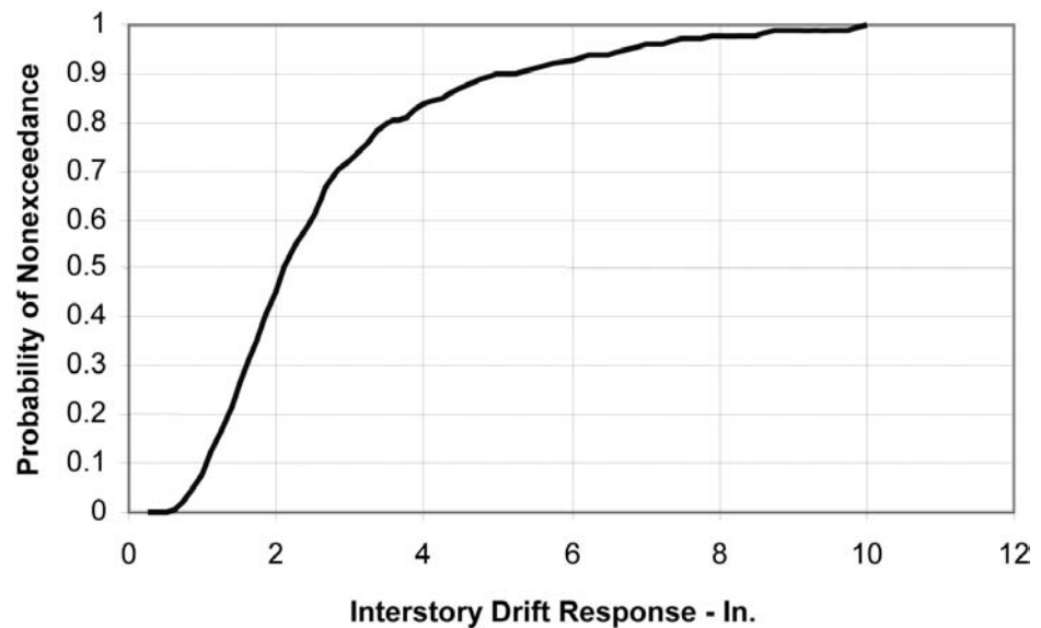
Figure B-3 Cumulative probability distribution for interstory drift response, conditioned on the 10%/50 year scenario event.
