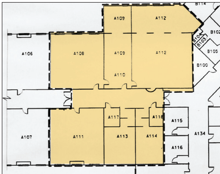
Figure 5-1: Diagram of the unventilated shelter area, which includes restrooms and drinking fountains, in an elementary school
