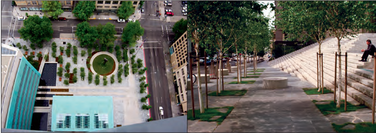
Figure 2-31: Use of planting to soften and enhance the appearance of walls and other security elements at the Seattle Courthouse
