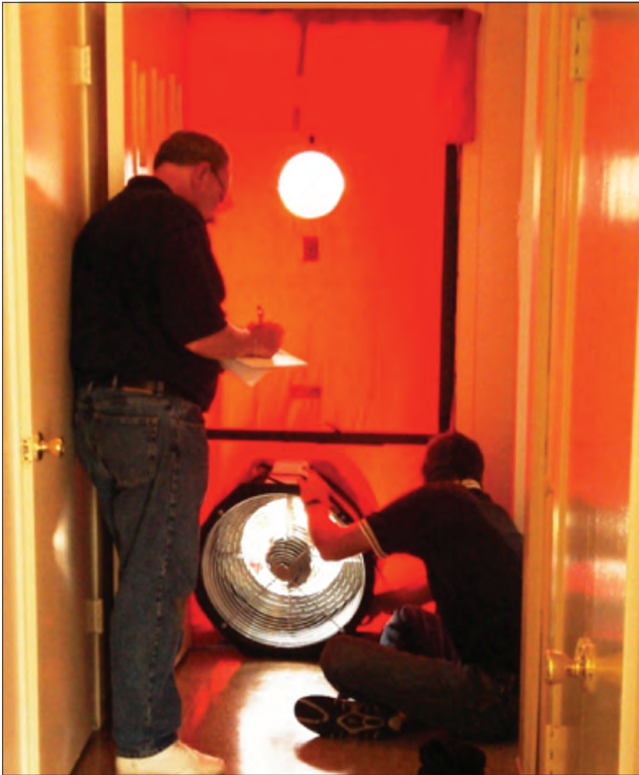
Figure 4-6: Blower door testing
